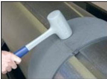
The second hammer blow should be delivered as pictured above, roughly in the center just above the seam.
