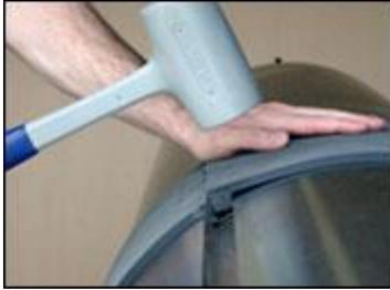
**Important:** Press lock bar end into keyway before striking it with dead-blow hammer.
