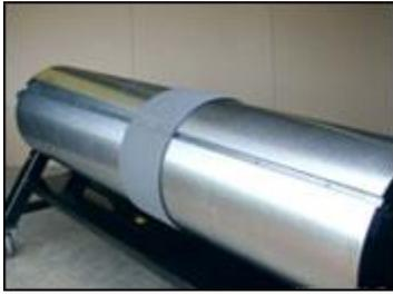
Always begin installation of the first TIMESAVER blankets at the center of the anvil cylinder.
