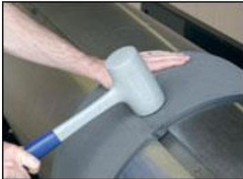
The first hammer blow should be delivered as pictured above, roughly 3 inches from the edge and just above the seam, with force.
